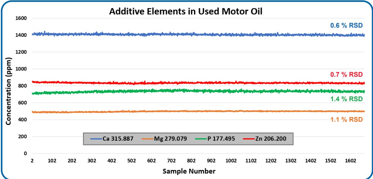
SampleSense Oil System 11+ hour stability run on iCAP PRO XPS for 4 additive elements
